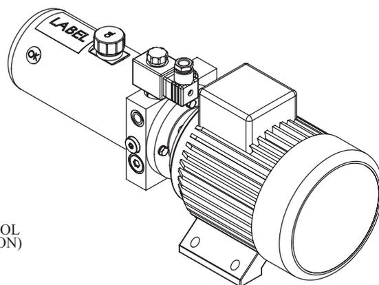
The W81AB mini power pack series is designed for use with European standard B14 AC motors.
